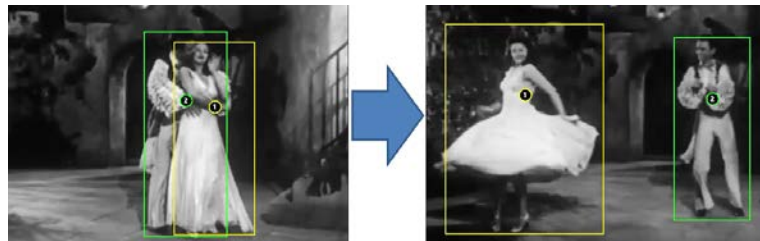
Figure 1. Automated tracking of subject motion using a Discriminative Scale Space Tracker.
